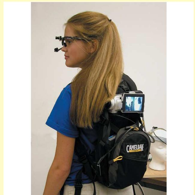
**Figure 1.** Portable, head mounted eye-tracker developed by Pelz and colleagues [15], based on commercially available systems that use an infrared video camera to image pupil and the corneal reflection. A camera mounted on the frame of the glasses records the scene from the observer's viewpoint. Eye position is then superimposed on the video record.
