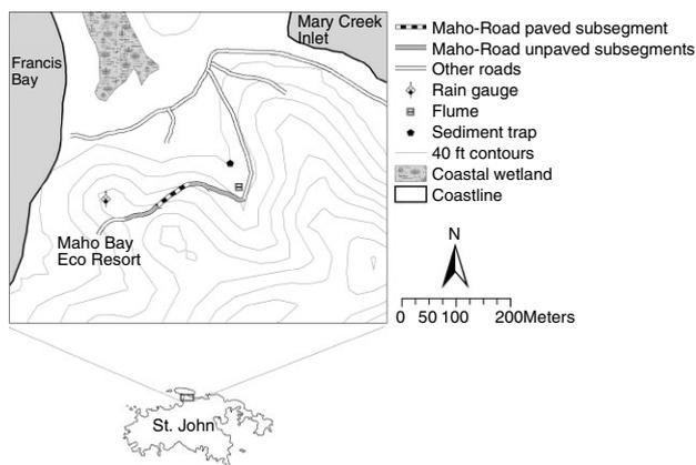
Figure 1. Map of the Maho Bay area showing the road segment that was studied and the location of the rain gauge, cutthroat flume, and sediment trap
