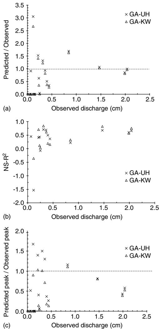
Figure 6. Performance of the GA-UH and GA-KW models for the 18 storms used for validation. (a) Observed discharge versus the ratio of predicted to observed discharge. The dotted line indicates perfect agreement. (b) Nash–Sutcliffe coefficient of determination  $R_{NS}^2$  versus total discharge. (c) Ratio of predicted to observed peak runoff rates versus total discharge. The dotted line indicates perfect agreement
