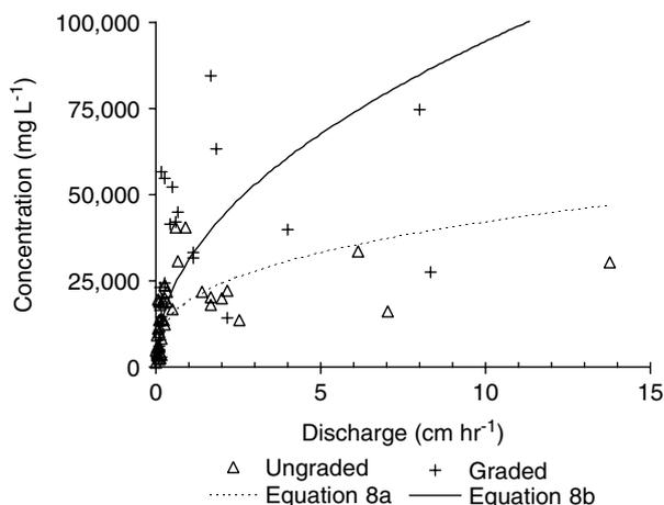
Figure 9. Relationship between suspended sediment concentrations and discharge for Maho-Road. Maho-Road was graded on 10 September 1999, and the data from 12 September to 25 October 1999 are plotted using a plus sign
