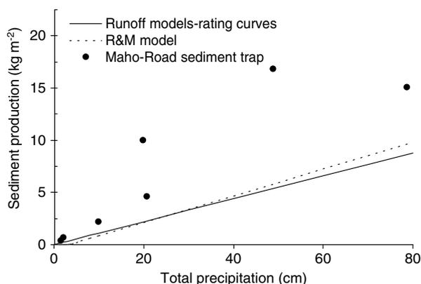
Figure 11. Relationship between total precipitation, measured sediment production rates using the sediment trap below Maho-Road, and predicted sediment production using the GA-UH model, GA-KW model, and R&M empirical road-segment model, respectively
