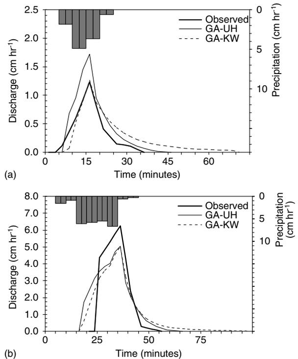
Figure 7. Hyetograph, observed hydrograph, and simulated hydrograph for: (a) 0.91 cm storm on 8 September 1999; (b) 2.36 cm storm on 5 January 2000
