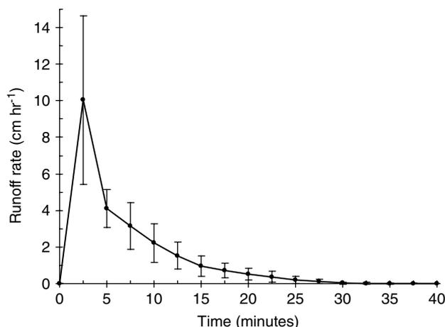
Figure 5. Mean 2.5 min UH for 1.0 cm of excess precipitation from Maho-Road. Bars indicate one standard deviation
