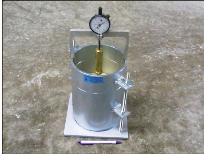
*Figure 4.21 Test Apparatus for Compacted CC Expansion Samples*
