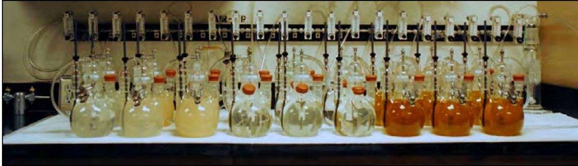
Figure 7.6 Purging of corrosion cells with oxygen during the STT.
