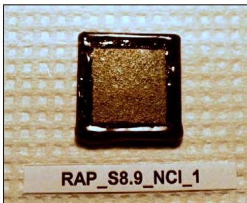
Figure 7.3 Typical steel sample following preparation for STT.
