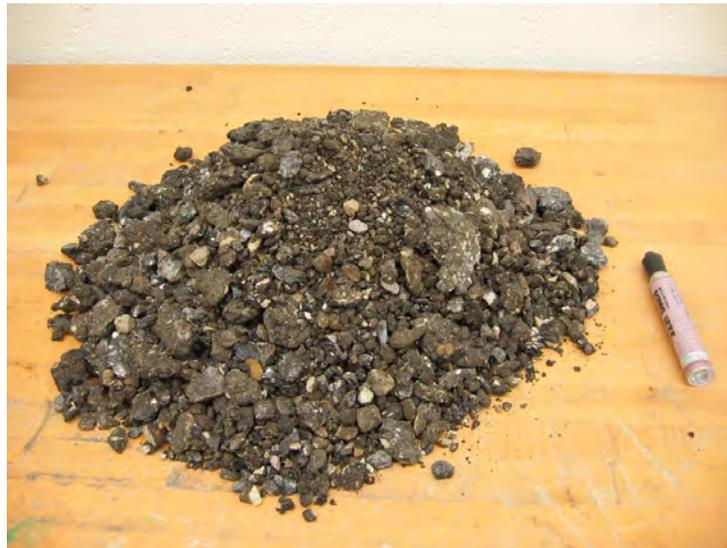
*Figure 2.2 Sample of Recycled Asphalt Pavement (RAP)*
