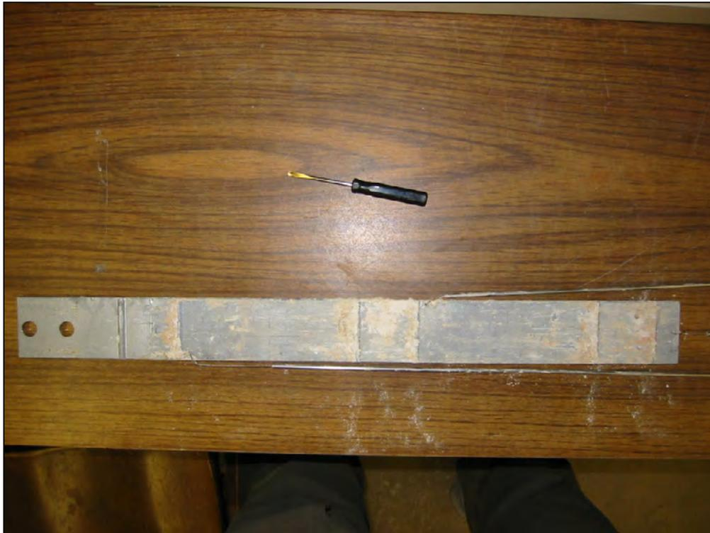
*Figure 5.2 Metallic ribbed strip reinforcement with sheathed telltales*
