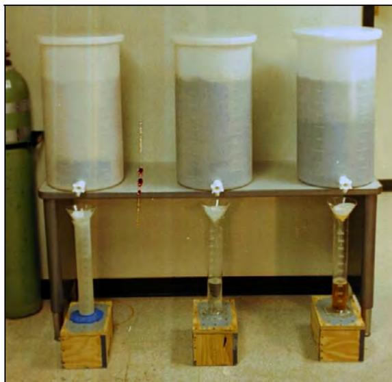
*Figure 7.5 Drainage collection from the backfill materials for the STT.*
