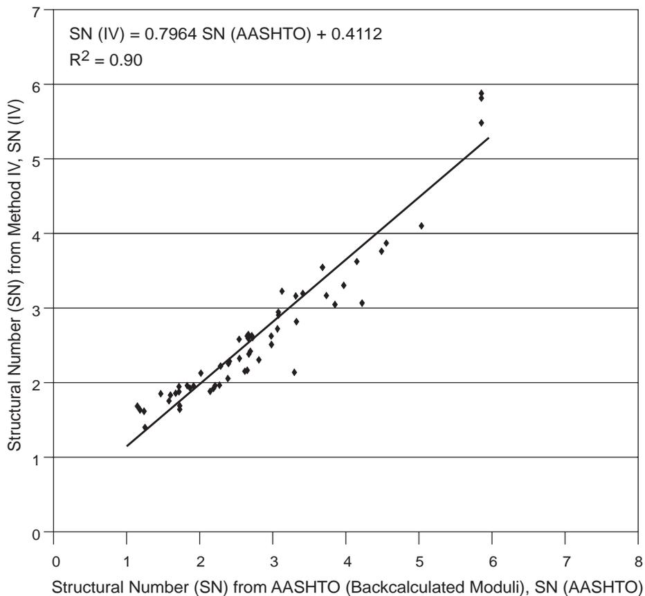
*Figure 4.2 Relationship of SN Using Method IV and SN Using Backcalculated Moduli for Selected ID Sections*
