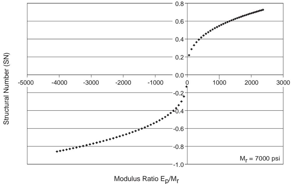
Figure 3.5 Relationship of Pavement Modulus and Structural Number in Method III
