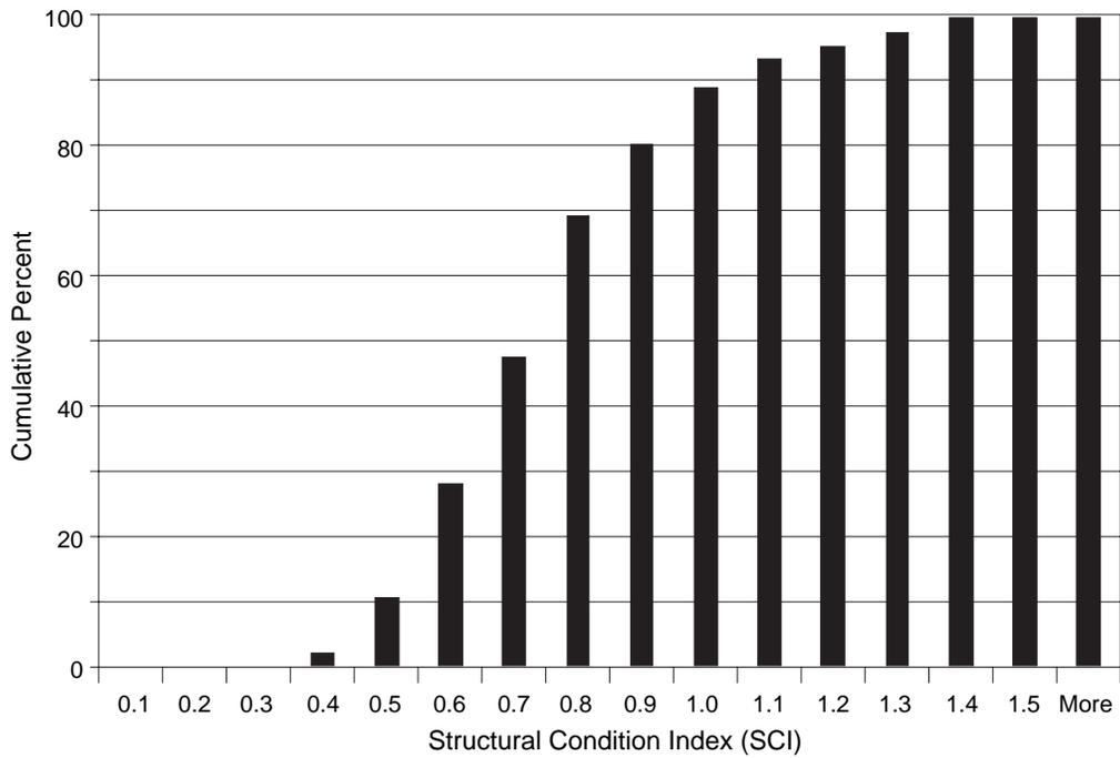
Figure 8.6 Cumulative Distribution of the SCI Values for the FM 762 Middle Subsection
