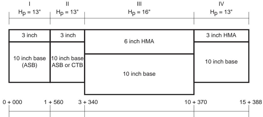
Figure 8.1 The Pavement Structures of the Subsections for FM 762
