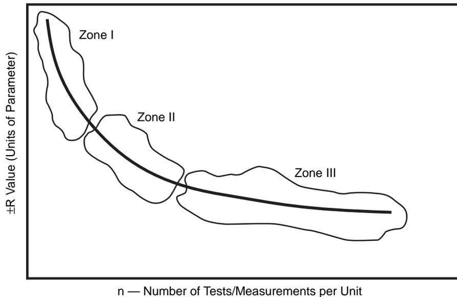
*Figure 6.2 Typical Limit of Accuracy Curve for All Pavement Variables Showing General Zones [AASHTO 1993]*
