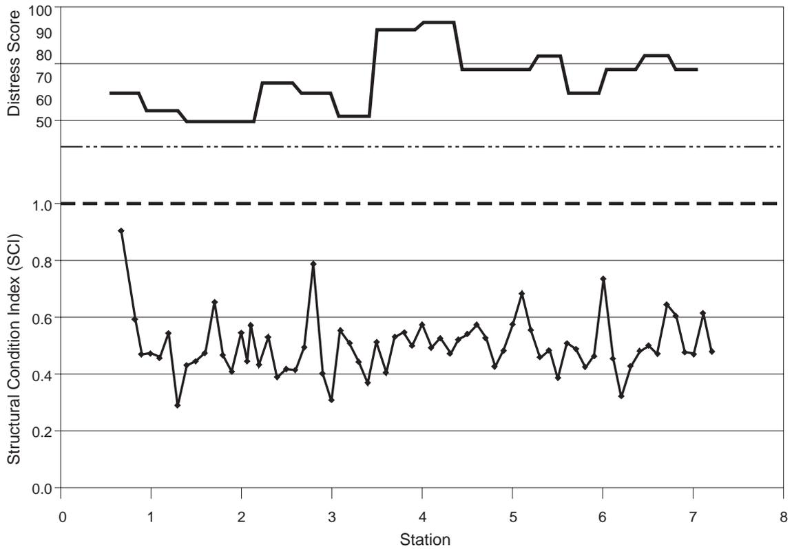
Figure 8.7 The SCI and Distress Scores for Section FM 1463
