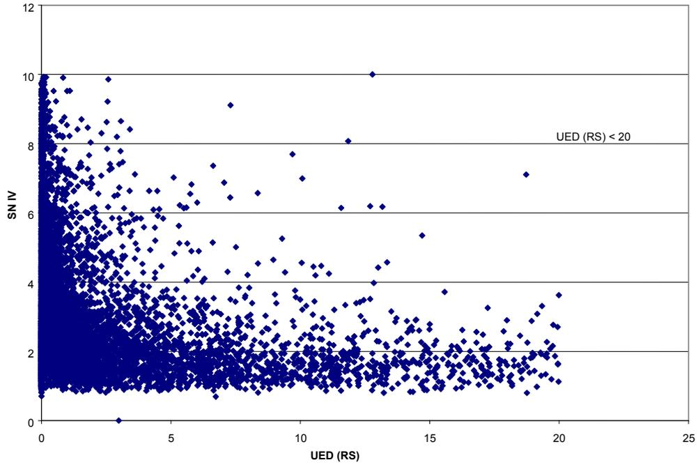
Figure B.9. Sensitivity of SN from Method IV to the UED of Ride Score, When Less Than 20
