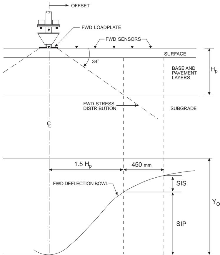
Figure 2.1 Stress Distribution and Measured Deflection Bowl Beneath FWD Load [Rohde 1994]
