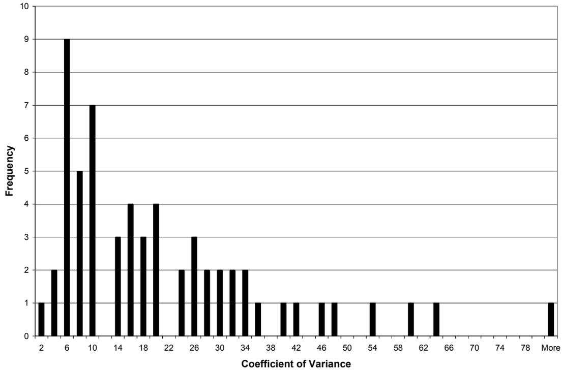
Figure 6.3 Histogram of the CV for 60 Sections Considered in the Analysis
