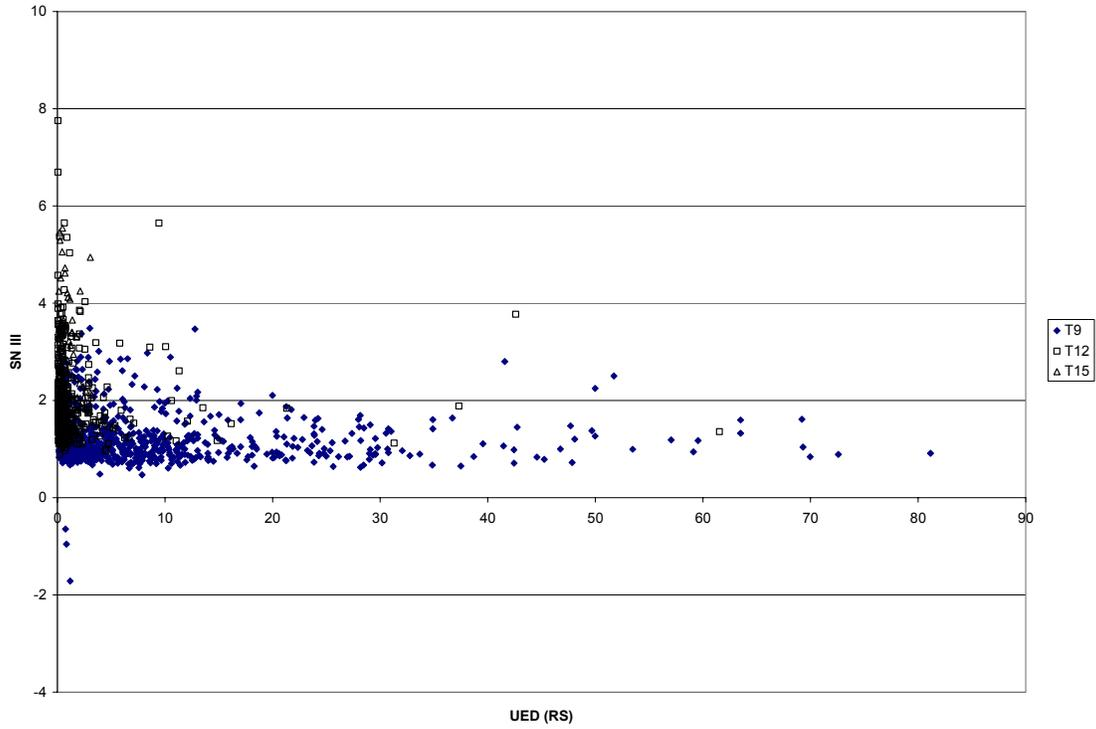
Figure A.17. Sensitivity of SN from Method III to the UED of Ride Score Stratified by Thickness
