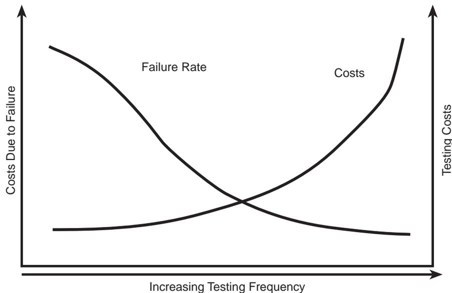
Figure 6.1 The Trade-Off Between Testing Costs and Failure Rate
