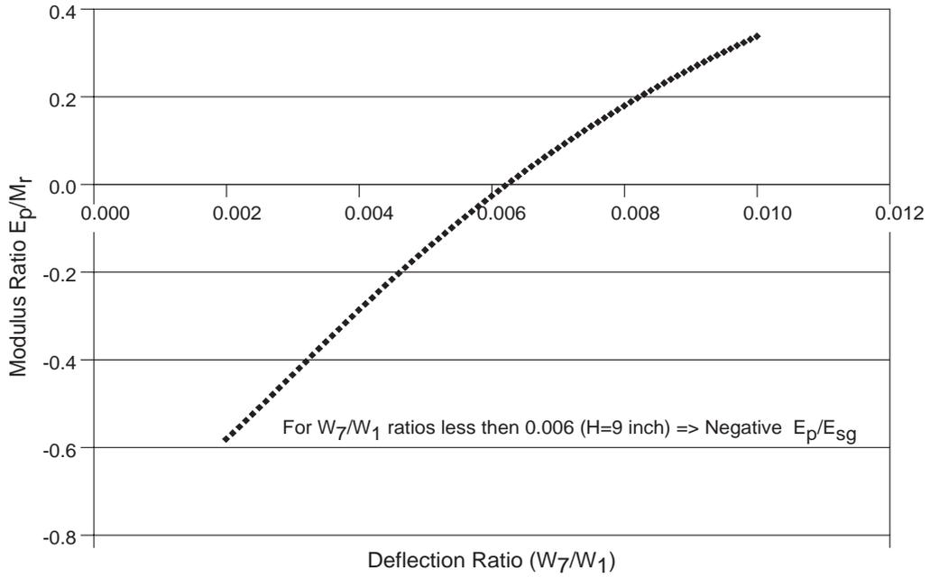
Figure 3.4 Relationship of the Deflection Ratio ( $W_7/W_1$ ) and Modulus Ratio  $E_p/M_r$
