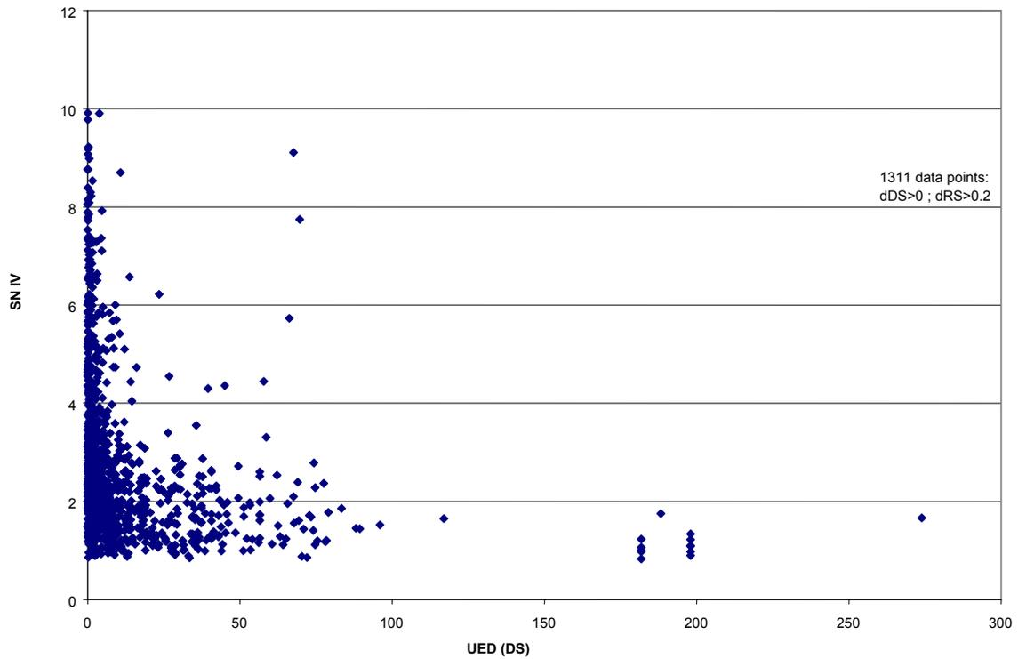
Figure B.12. Sensitivity of SN From Method IV to the UED of Distress Score, When dDS Greater Than 0 and dRS Greater Than 0.2
