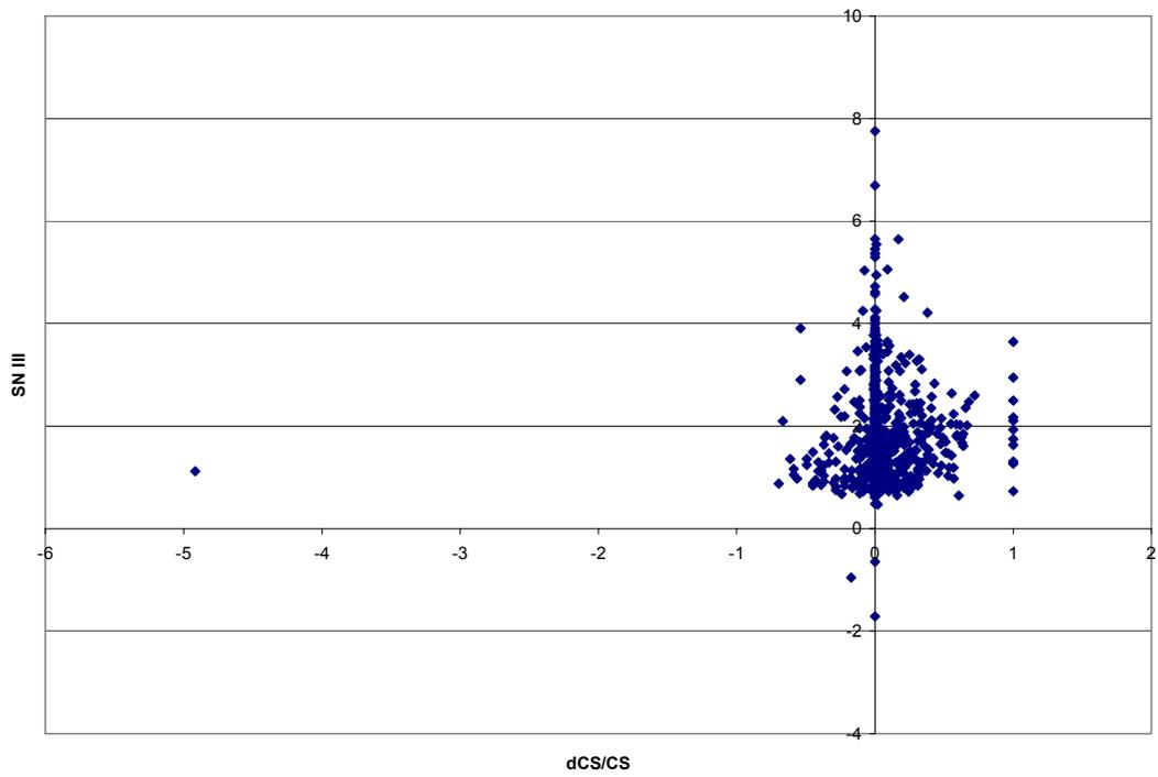
Figure A.2. Sensitivity of SN from Method III to the Yearly Change in Normalized Condition Score
