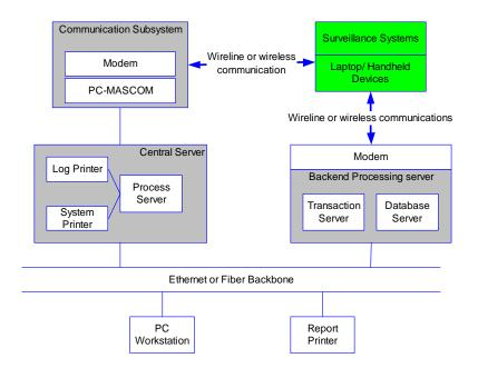
*Figure 2-1. Typical communications between surveillance systems and TMC servers.*
