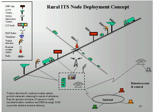
Figure 2-3. Rural ITS node deployment concept.
