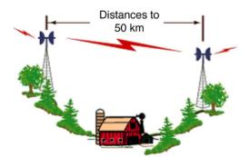
Figure 3-2. Maximum distance between base stations for fixed wireless technology (Rysavy, 2002).
