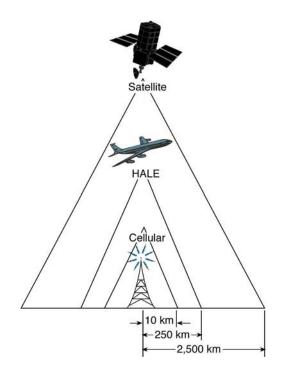
Figure 3-3. Service range of three types of wireless communication technologies (Rysavy, 2002).
