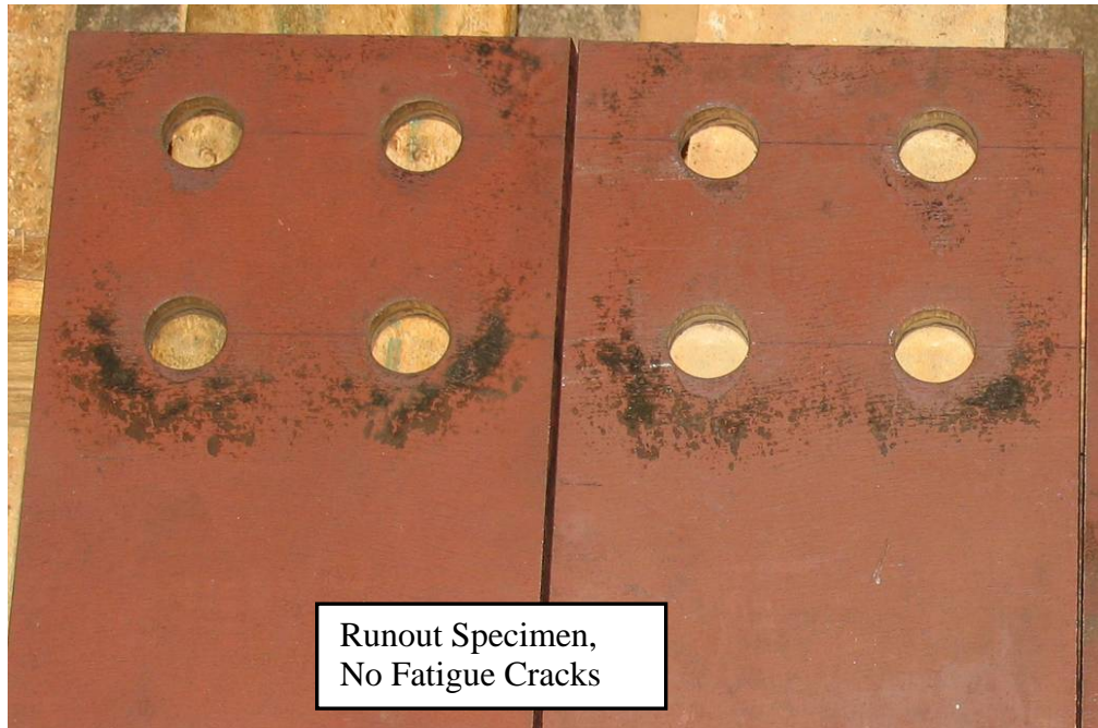
Figure 4.35: Typical Pretensioned Bolt Connection Fatigue Runout Specimen Surfaces, N=3,611,171+
