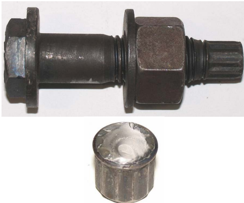
Figure 3.39: 7/8 in. A490 Twist-Off Type Bolt Used for Tests
