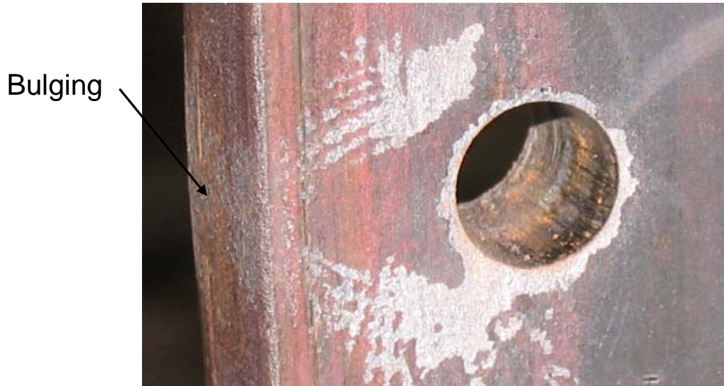
Figure 4.15: Example of bulging from hole punching
