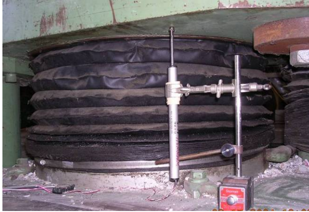
Figure 3.30: Linear Potentiometer at Base of UTM
