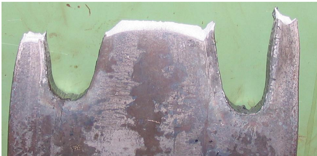
Figure 4.51: Single plane failure of A36 steel specimen
