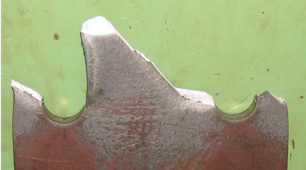
Figure 4.49: Typical failure for Grade 50 steel 3/8" plate
