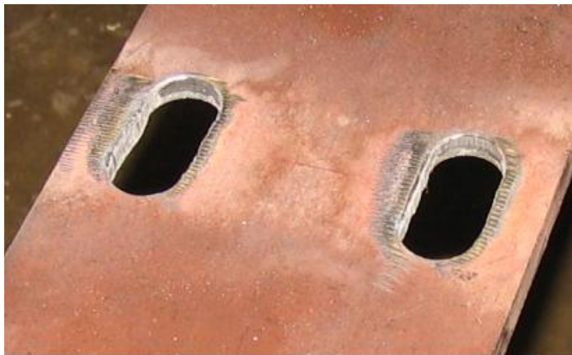
Figure 3.4: Phase 2 of making of slotted holes
