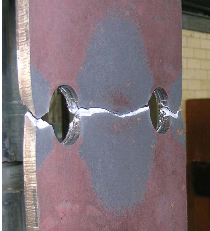
Figure 4.2: Typical Failed Punched Hole Plate Specimen
