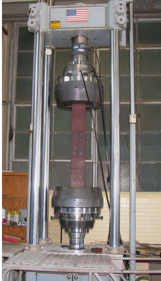
Figure 3.31: FSEL 220-kip MTS Load Frame, Shown with Connection Specimen
