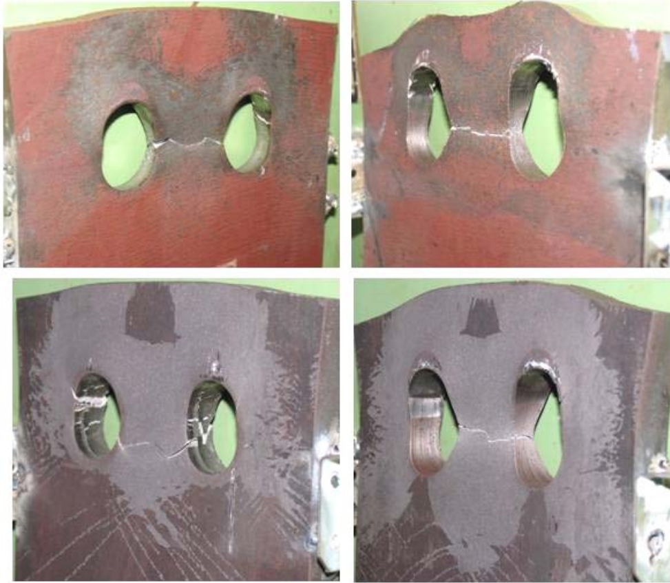
Figure 4.21: Experimental Block Shear Type Failures
