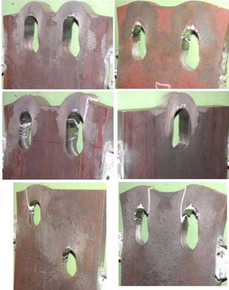
Figure 4.22: Experimental Bearing Type Failures
