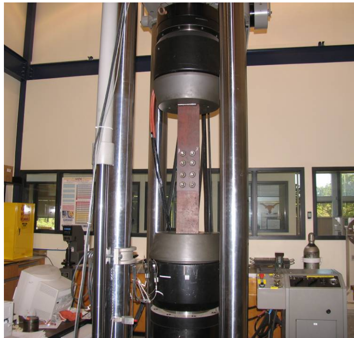
Figure 3.43: TxDOT 550 kip MTS Load Frame, Shown with Connection Specimen
