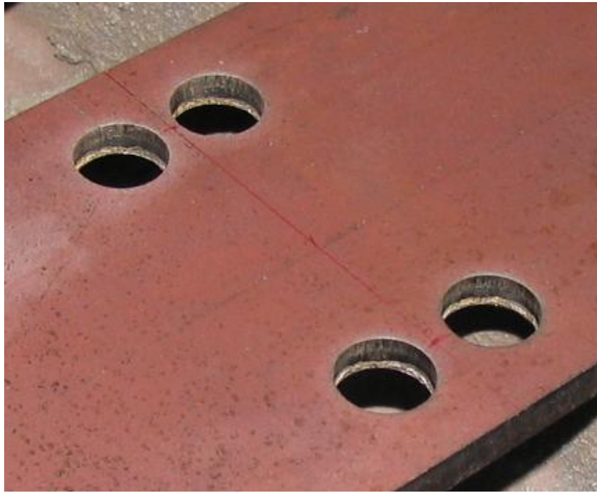
Figure 3.3: Phase 1 of making slotted holes
