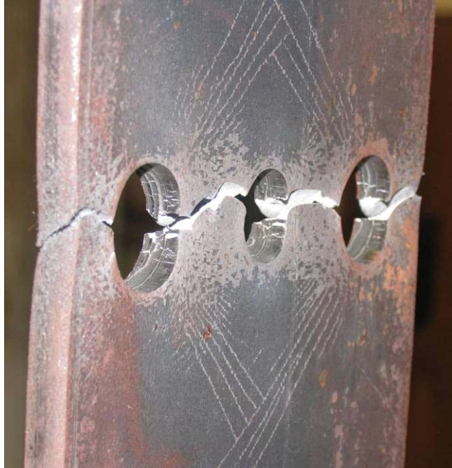
Figure 4.4: Reduced Net Area Plate Specimen Failure—Punched Holes
