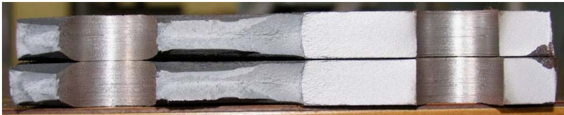
Figure 4.11: Cross-Section of A588—2 Sets of Drilled Holes Specimen at Failure; Worn Drill Bit Hole Line, N=710,415
