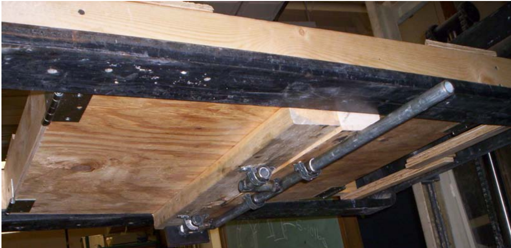
Figure 4.19: Drop Test Release Mechanism
