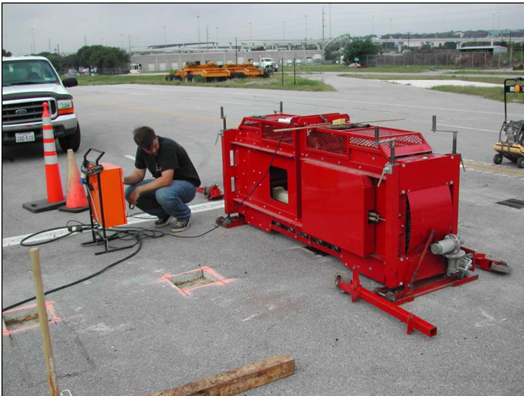
Figure 5.1: Model Mobile Load Simulator(MMLS3)
