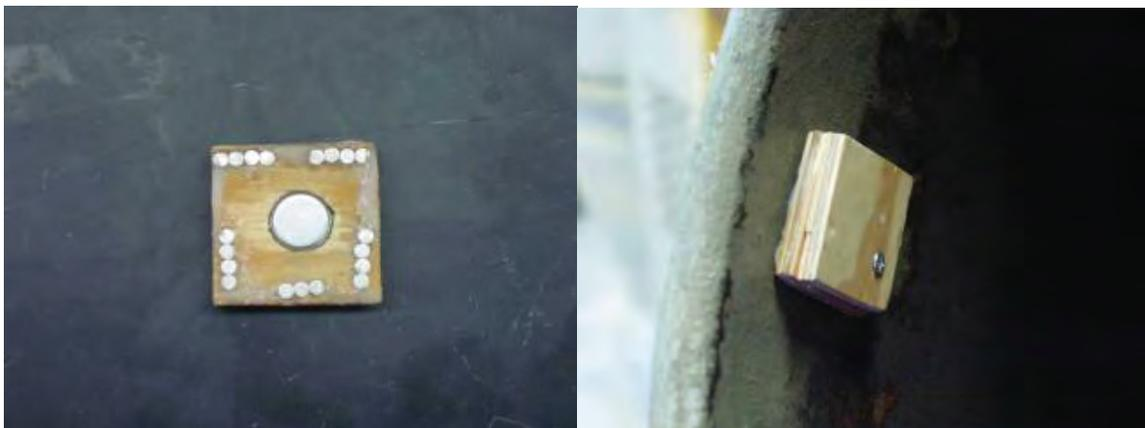
Figure 8.4 a. iButton temperature sensor in protective casing; b. iButton sensor attached to the side of a laboratory mixing drum
