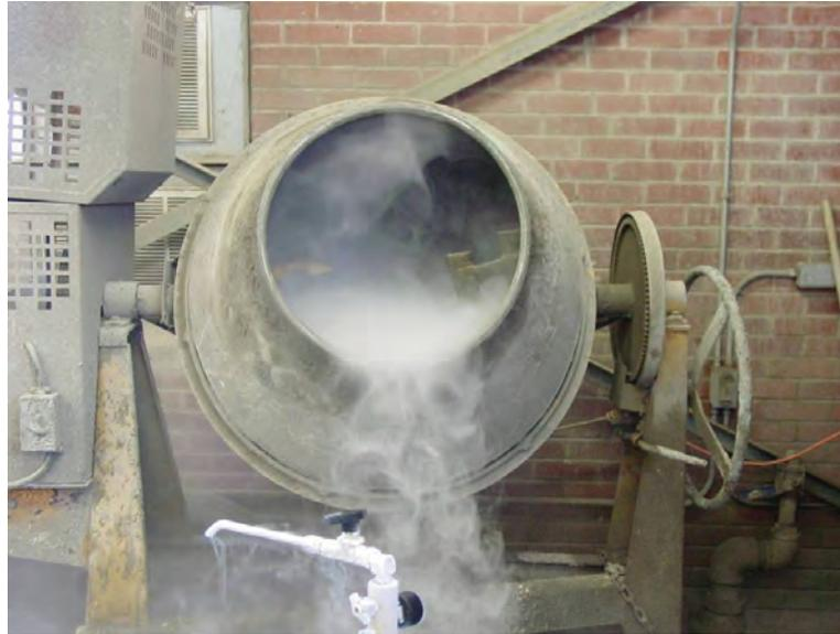
*Figure 3.3 Vapor flows freely from the uncovered mixer*
