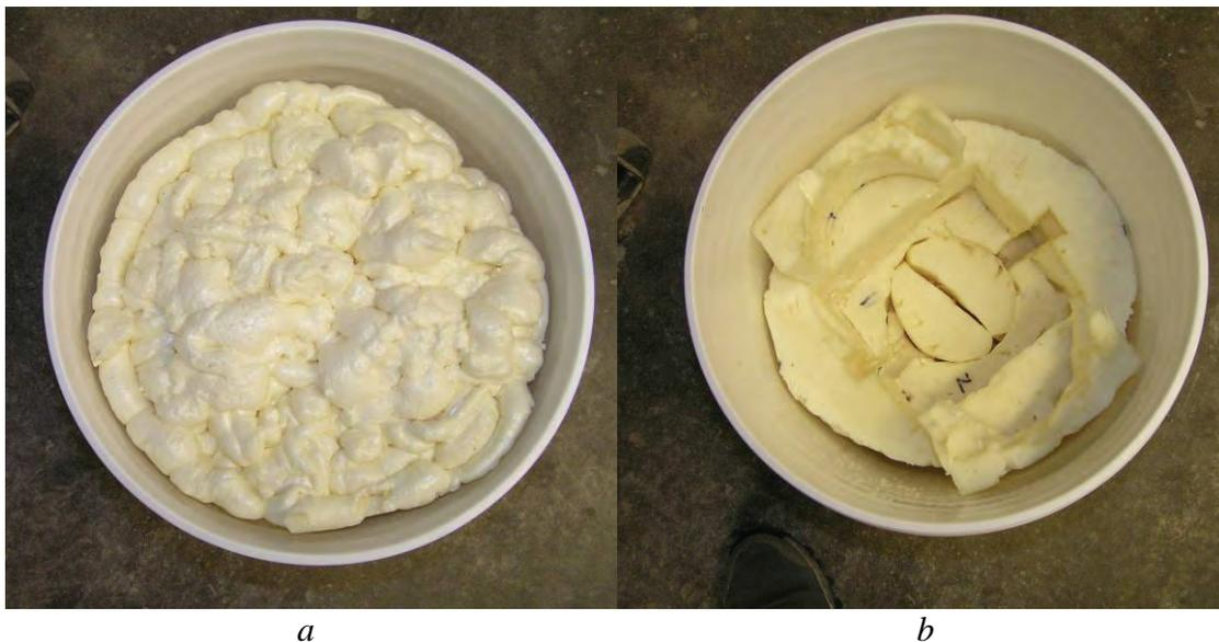
Figure 6.1 Insulating chambers made for set time specimens
