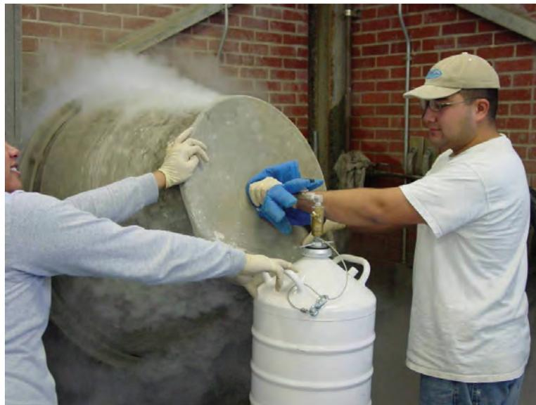
*Figure 3.4 Plastic cover with hole in the middle for liquid nitrogen dosing*
