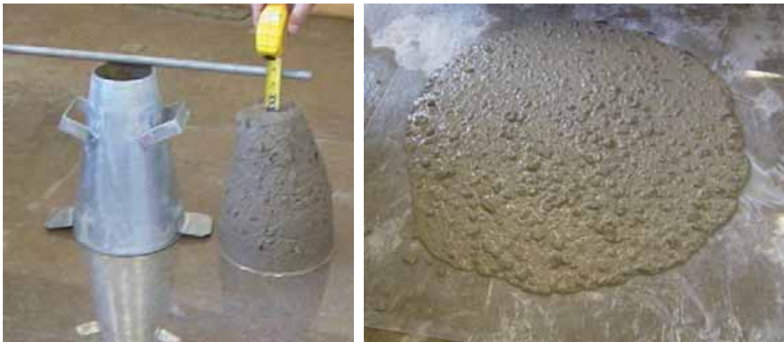
Figure 1.1: Flow Properties of Conventionally Placed Concrete (Left) and SCC after Removal of the Slump Cone
