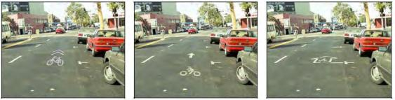
Bike-and-chevron markingBike-and-separate-arrow markingBike-in-house markingFigure 2.8: Photographs of Pavement Markings Used in Stated Preference Survey
