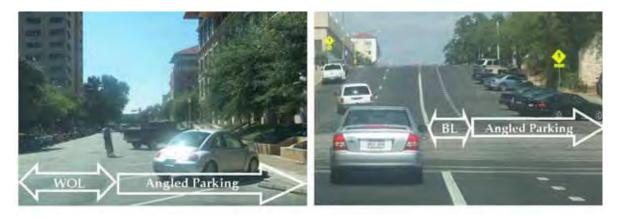
Figure 3.3: Examples of angled motor vehicle parking adjacent to a BL (right) and WOL (left)
