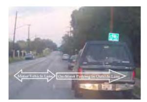
*Figure 3.6: Example of bicycle route with parking in the outside lane*
