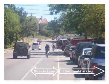
*Figure 3.1: Example of a bicycle lane with adjacent on-street motor vehicle parking*
