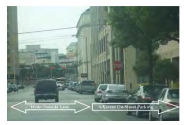
Figure 3.2: Example of a wide outside lane with adjacent motor vehicle parking
