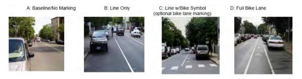
Figure 2.7: Added Components of Bicycle Lane
