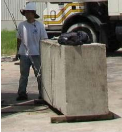
Figure 2.3.8 – Tie down tied to concrete block
