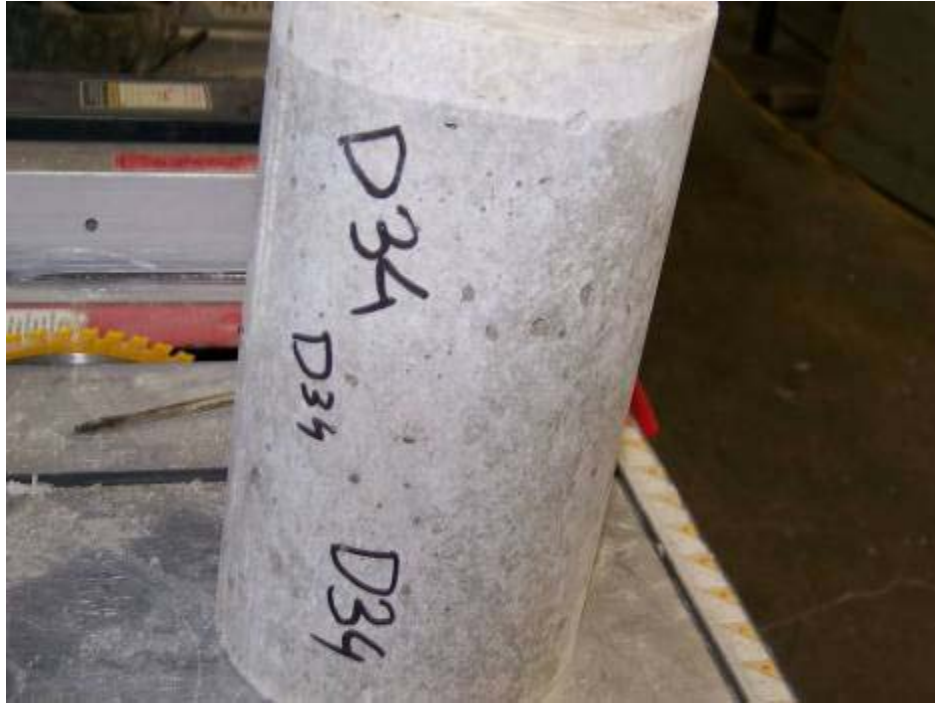
Figure 2.4.5 – UCS Sample obtained from 6" PVC pipe
