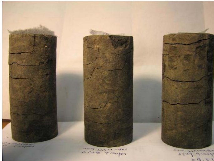
Figure 1.5.56 Outlook of Navarro Shale specimen during drying
