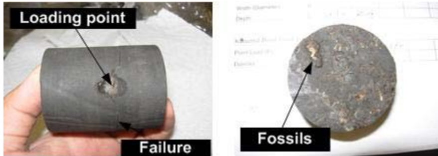
Figure 1.4.20 Failed specimen by diametral point load test
