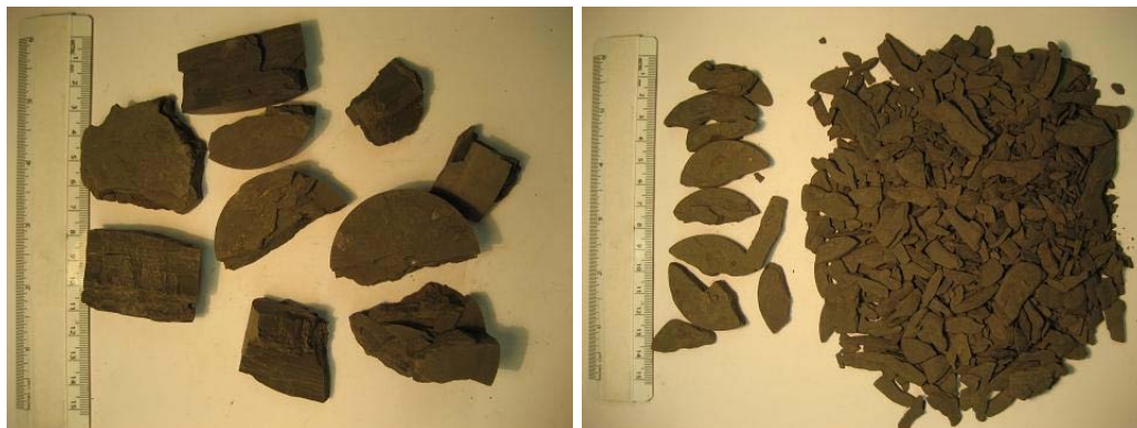
Figure 1.5.38 Eagle Ford Shale before and after the slake durability test (EFMSN)
