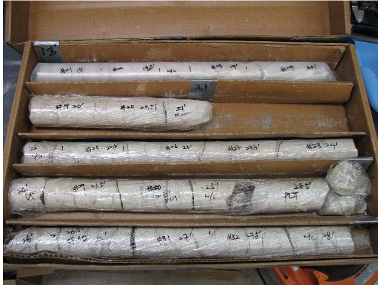
Figure 1.5.1 Edwards limestone cores before specimen preparation
