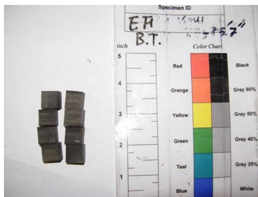
Figure 1.3.8 Half inch cubic shale samples of Eagle Ford Shale
