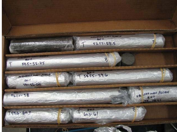
Figure 1.5.55 Navarro Shale cores prior to sample preparation
