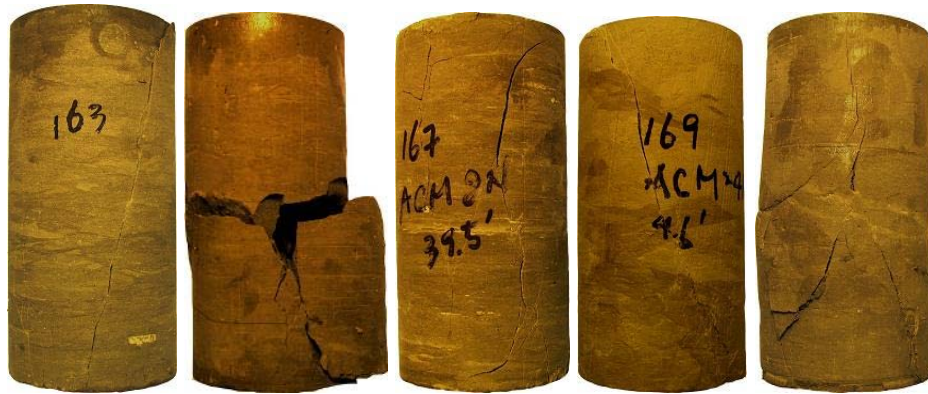
Figure 1.5.13 Failure modes of Austin Chalk after the multi-stage triaxial test
