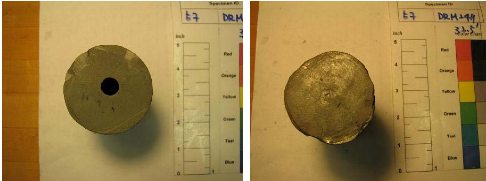
Figure 1.5.25 Holed Del Rio Clay specimen before and after the multi-stage triaxial test
