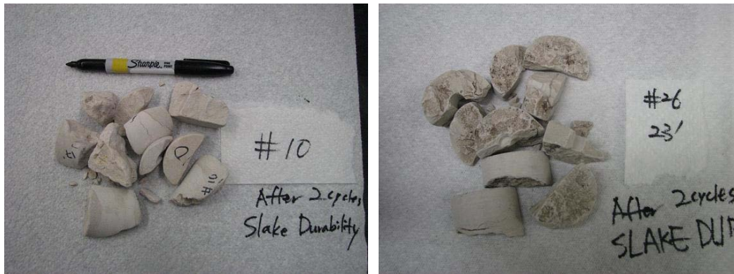
Figure 1.5.5 Edwards Limestone specimens after slake durability tests
