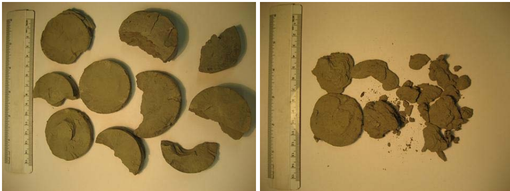
Figure 1.5.26 Del Rio Clay before and after two cycles of the slake durability test (DRM48N)
