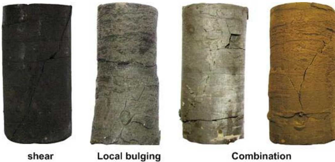
Figure 1.5.47 Failure modes of Taylor Marl after the multi-stage triaxial test
