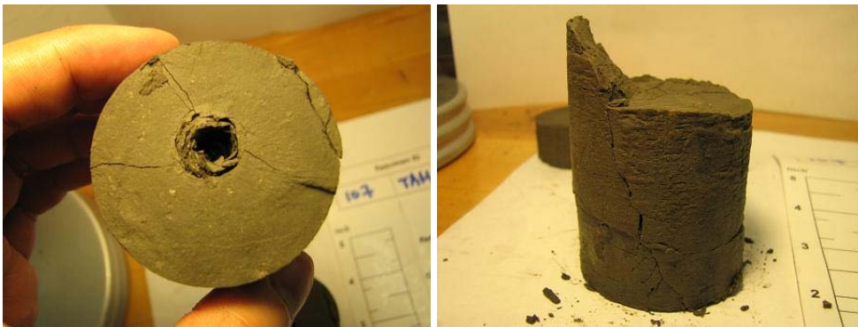
Figure 1.5.48 Holed Taylor Marl specimen after the triaxial test
