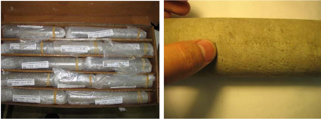
Figure 1.5.9 Austin Chalk cores before specimen preparation
