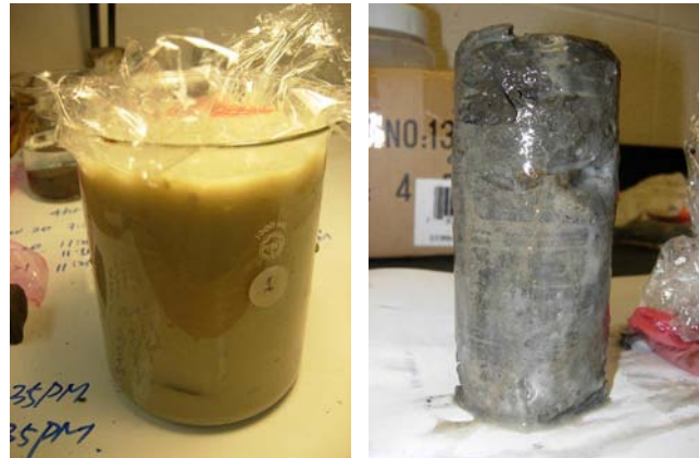
Figure 1.5.61 Slurry-soaked Navarro Shale specimen
