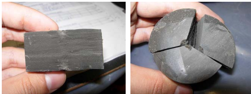
Figure 1.4.22 Failed specimens by axial point load test
