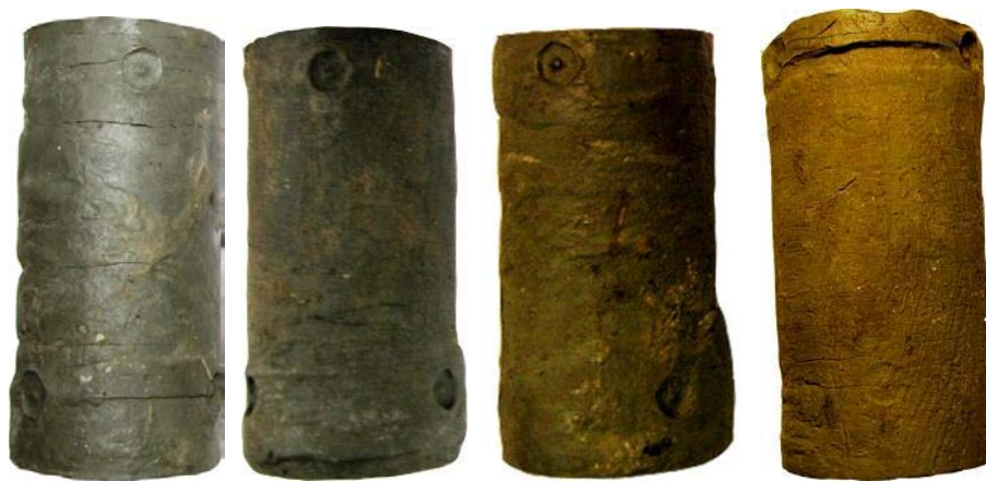
Figure 1.5.24 Failure modes of Del Rio Clay specimens
