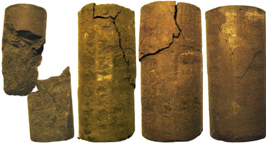
Figure 1.5.60 Failure modes of several Navarro Shale specimens
