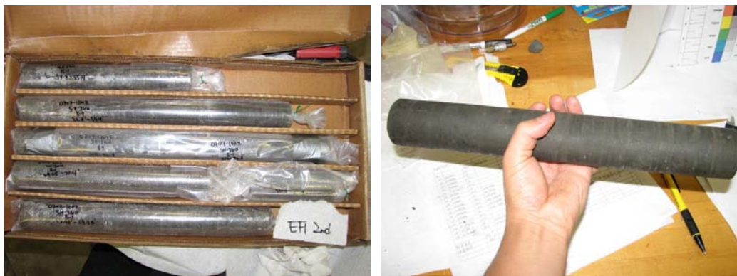
Figure 1.5.32 Eagle Ford cores prior to sample preparation
