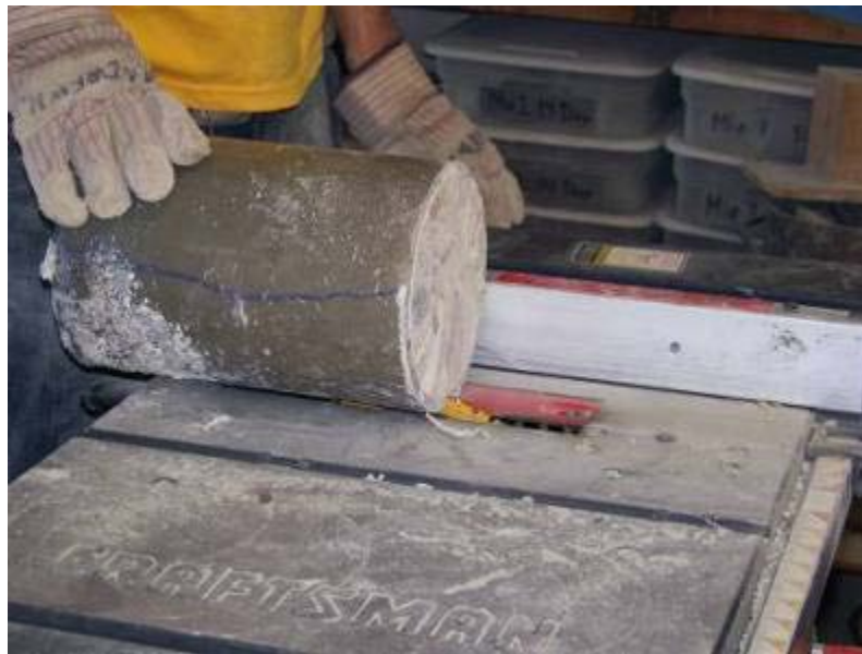
Figure 2.4.4 – Concrete cylinder extracted by cutting the clear PVC pipe
