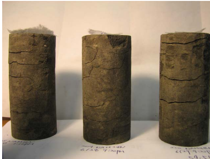
Figure 1.4.7 Developed fissures of dried Navarro Specimens
