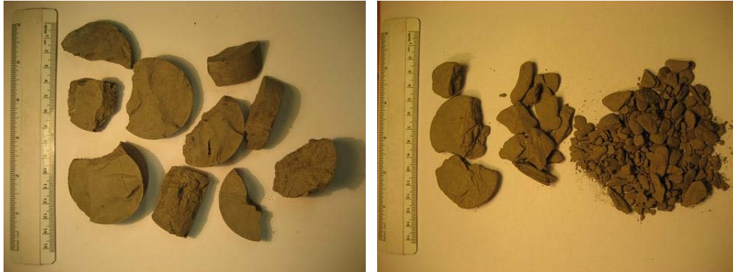
Figure 1.5.50 Taylor Marl before and after the slake durability test (TAM4N)
