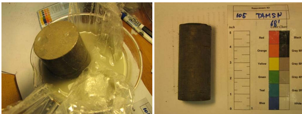
Figure 1.5.49 Taylor Marl slurry-soaked for 12 hours
