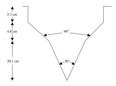
Figure 4.3 Compound V-Notch Weir for Flow Measurement
