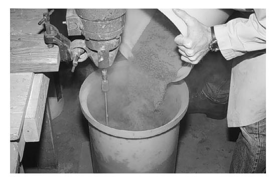
Figure 3.4 Addition of Sediment and Clays for Creation of Highway Runoff Cocktail
