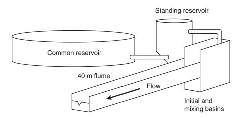
Figure 3.3 General Flume Apparatus
