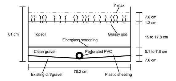
Figure 3.1 Cross Section of Channel Swale
