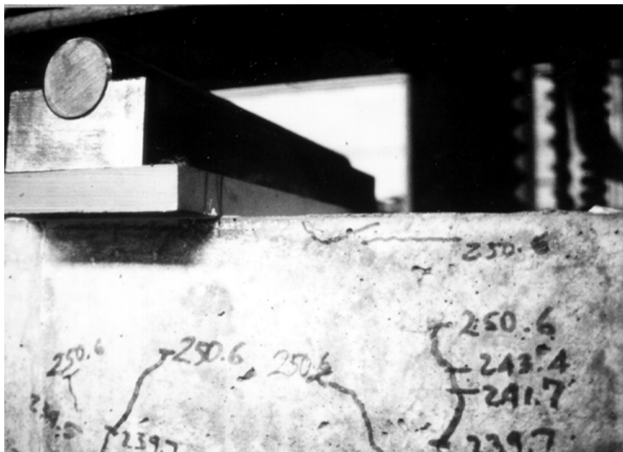
Figure 4.13 Local concrete crushing (Test 2-DIS-119)
