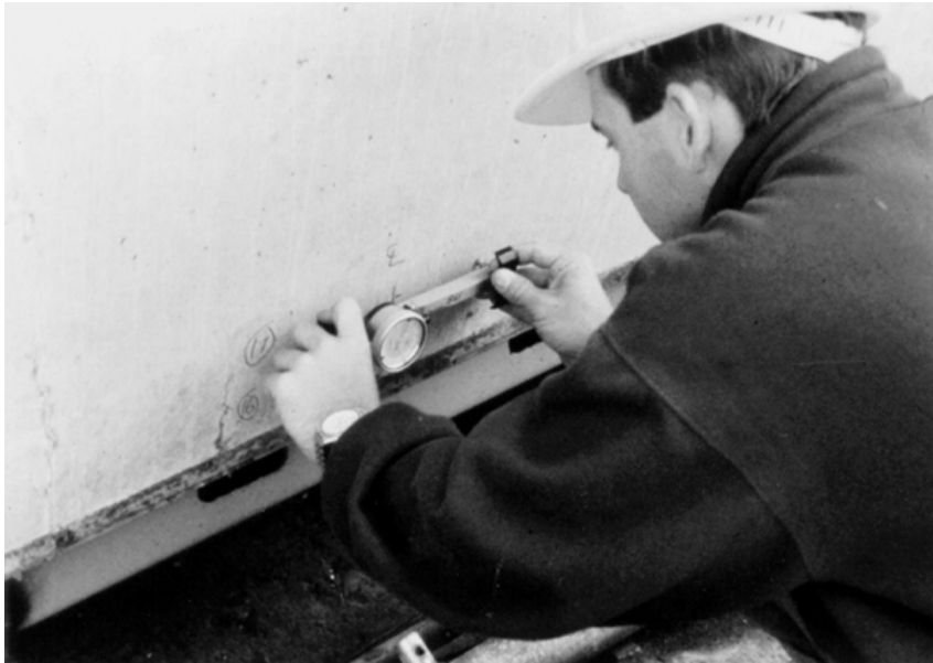
Figure 3.5 Reading of DEMEC points
