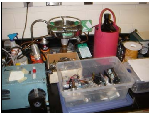
Cluttered workspace. Emergency eyewash obstructed.
