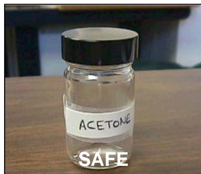
Properly labeled secondary storage container
