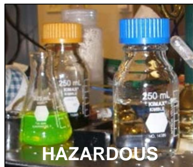
Improperly labeled secondary storage container
