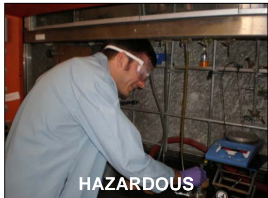
Improper use of the fume hood
