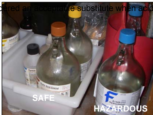
Proper and improper acid storage methods
