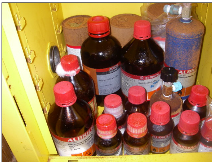
Chemical containers in poor condition from corrosion and crystal formation.
