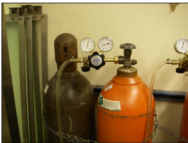
Properly attached regulator and safety cap
