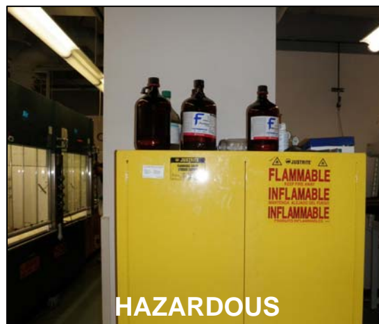
Improper storage of chemicals above eye level
