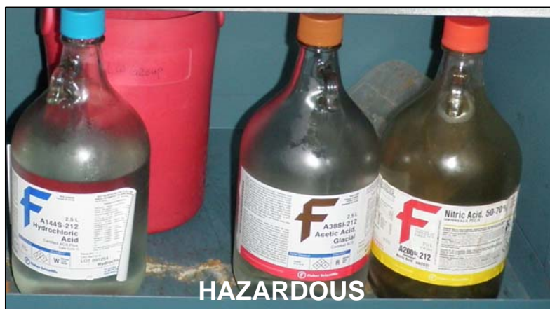
Improper storage of nitric acid
