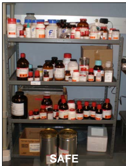
Proper storage of chemicals below eye level
