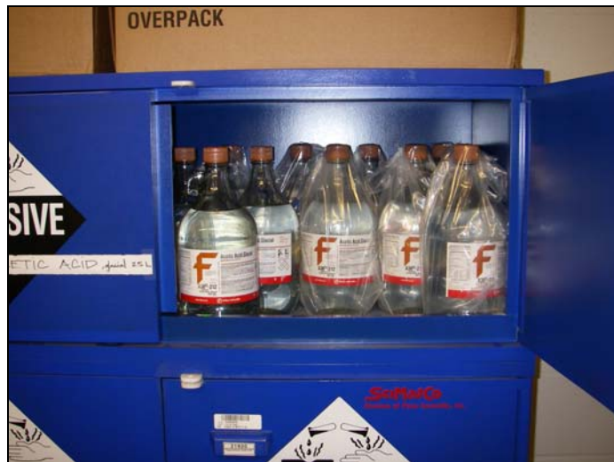
Acids stored in acid storage cabinet
