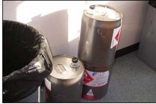
Improper storage of flammable chemicals
